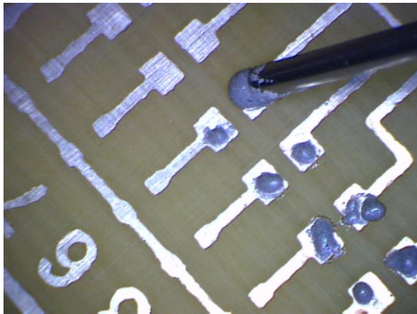
Figure 2H: Applying solder paste from a syringe
