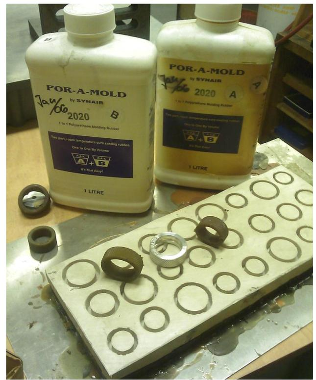
measure carefully when mixing Part A and Part B to ensure you have a 1:1 ratio. "Eyeballing" it is insufficient, and will produce sticky, messy wheels that don't set up properly. I have used syringes, while BCIT's master tire caster, Eugene Duruisseau, uses small measuring cups. You'll have about five minutes of working time with the resin, once mixed, and should allow several hours for it to set.
